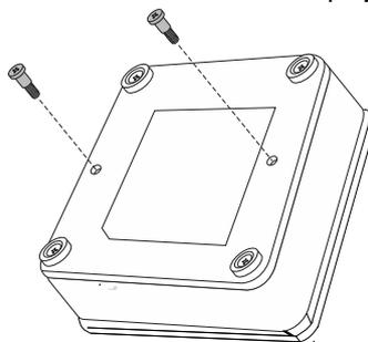
2. Fasten two screws to the bottom of VIA Connect<sup>2</sup>.
