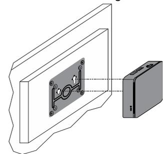
3. Insert the screws on the bottom of VIA Connect<sup>2</sup> into the slots on the mounting bracket.
