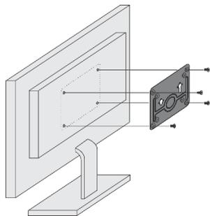
1. Attach the VESA mounting bracket to the back of the display with 4 screws.
