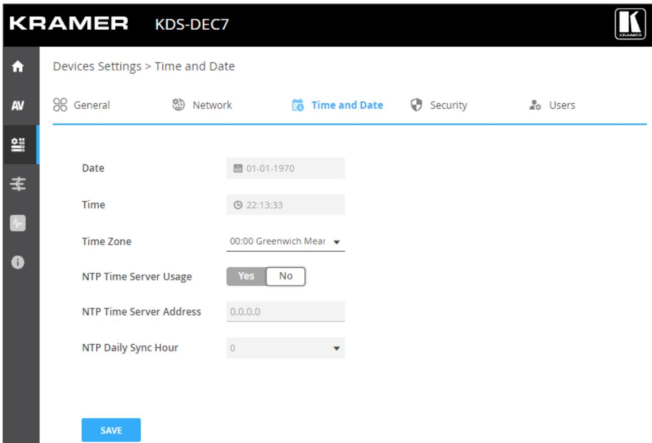
Figure 49: Device Settings Page – Time and Date Tab
