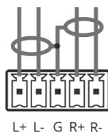
Figure 4: Connecting to a Balanced Stereo Audio Source/Acceptor
