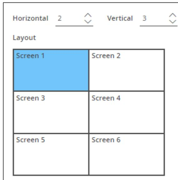
Figure 43: 2x3 Video Wall Configuration
