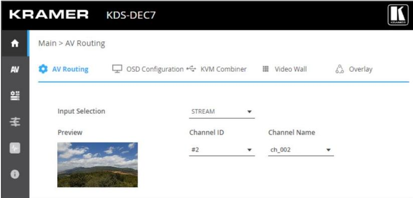
Figure 58: KDS-DEC7 Setting Channel ID and Name
