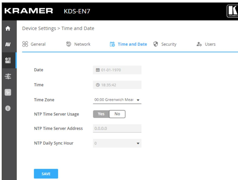
Figure 19: Device Settings – Time and Date Tab
