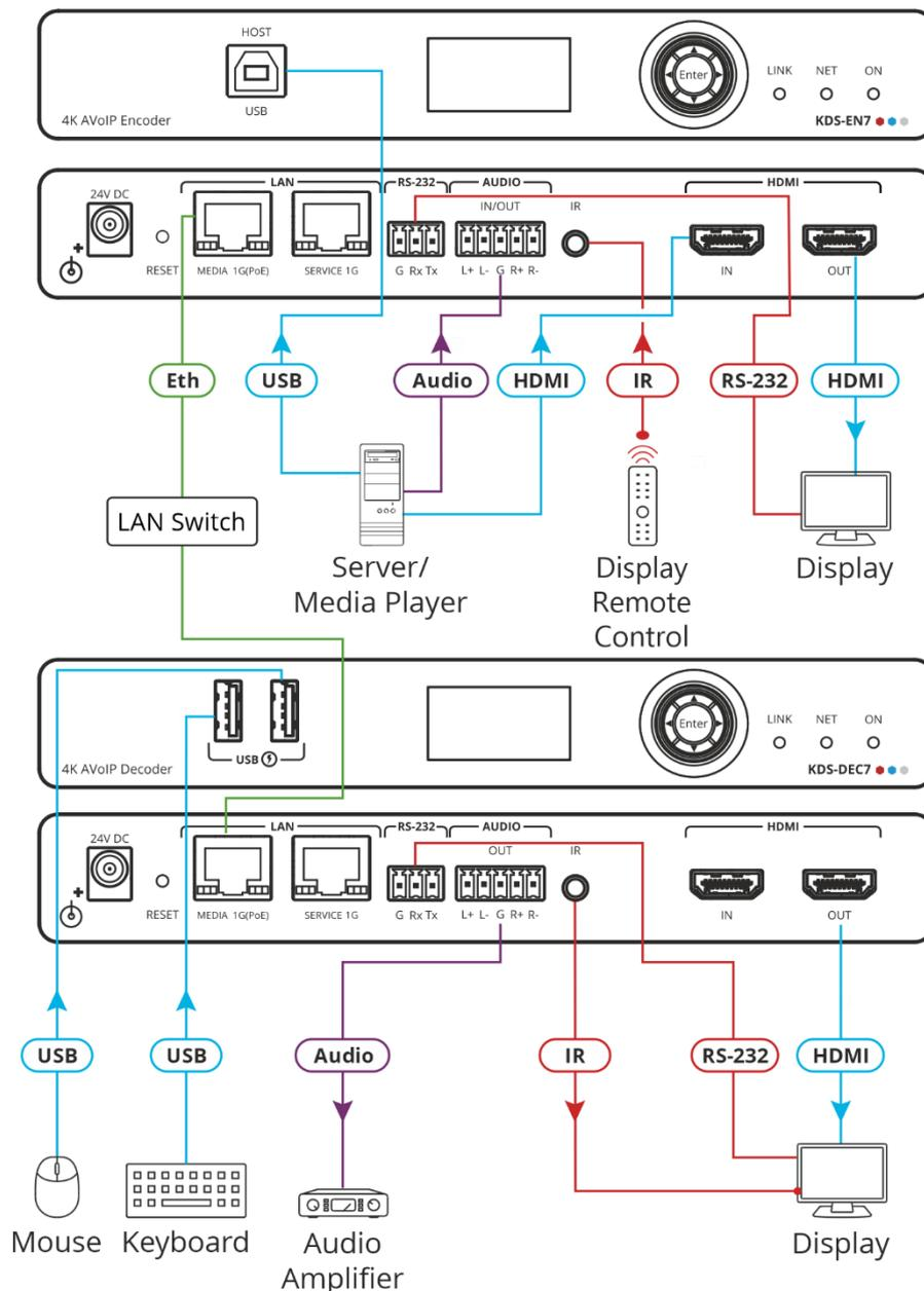
Figure 3: Connecting the KDS-EN7 and KDS-DEC7
