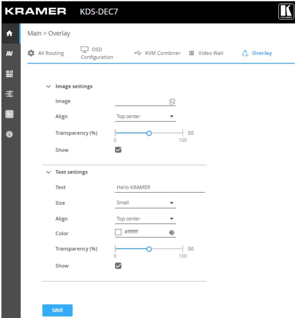
Figure 44: Main – Overlay Tab
