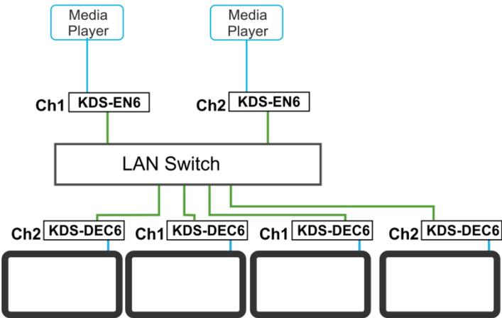
Figure 9: Connecting the KDS-EN6, KDS-DEC6 Video Encoder/Decoder
