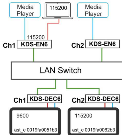
Figure 35: Serial over IP – RS-232 over IP
