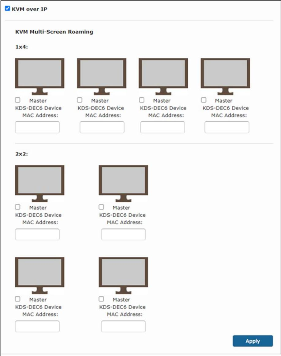
Figure 13: KVM Roaming Configuration
