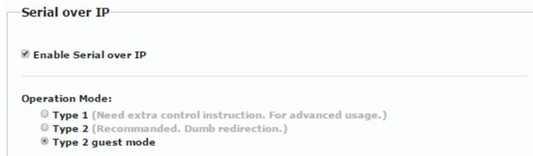
Figure 38: Serial over IP – Type 2 Guest Operation Mode
