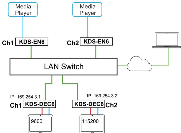
Figure 37: Serial over IP – Type 2 Guest connection
