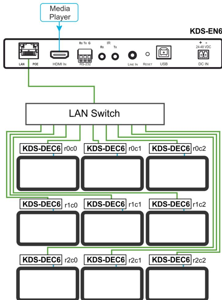
Figure 10: Video Wall Setup
