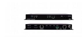
KDS-8 is a high-performance, zero latency, 4K@60Hz (4:4:4) video streaming transceiver for streaming via Ethernet over copper cable. KDS-8 can be set as either an encoder or decoder. As an encoder, it encodes and streams the HDMI input along with IR, RS-232, and analog audio, over an IP network. As a decoder, it receives the encoded signal and decodes it for output
