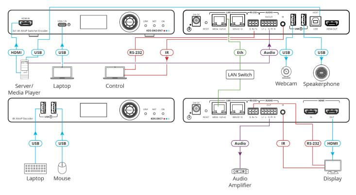
**KDS-SW2-EN7** and **KDS-DEC7** can stream 4K video, requiring a gigabit Ethernet switch for high quality performance, since the maximum momentary transfer rate can reach 850Mbps. We recommend using AVoIP Ethernet switches that support: Multicast forwarding or filtering, IGMP Snooping, IGMP Querier, IGMP snooping fast leave and Jumbo frame (8000 bytes or larger).
