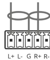
Figure 4: Connecting to an Unbalanced Stereo Audio Acceptor
