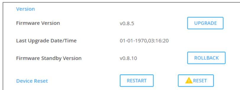
Figure 23: Device Settings Page – Firmware Upgrade
