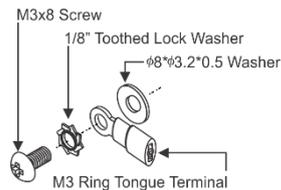
1. Connect the ring tongue terminal to the building grounding point wire (a green-yellow, AWG#18 (0.82mm<sup>2</sup>) wire, crimped with a proper hand-tool is recommended).
