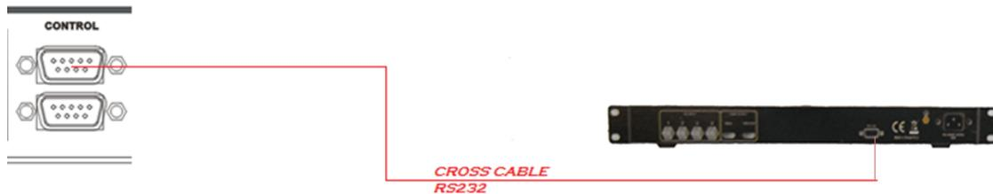
2. RS232 control conference tracking and recording all-in-one machine VIS-CRS05-A.
